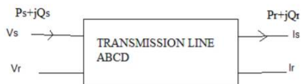
Figure 1: Two port four terminal model of a transmission line.
